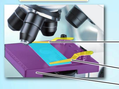
The stage is where you place the <u>slide</u> which contains the <u>specimen</u>.
